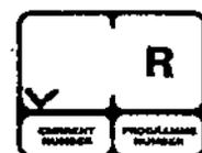
**Non remote control mode** with no 90 degrees reverse or forward function = Symbol **o**.
